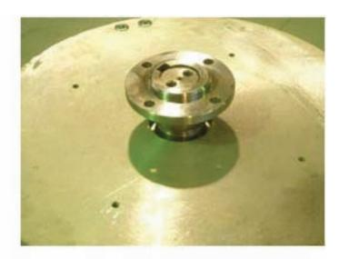
AFTER DISASSEMBLED BLADE SUPPORT, DISASSEM-BLY HUB
