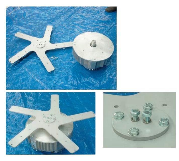
PLACE BLADE SUPPORT WITH DISC OVER THE SHAFT AND CLAMP SCREWS M10x35 TE WITH NUTS GROWER D.10
