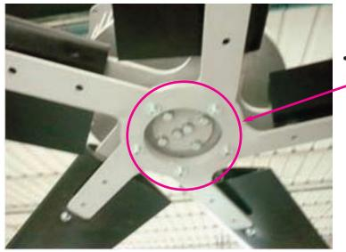
Fix without tightening the 5 central
