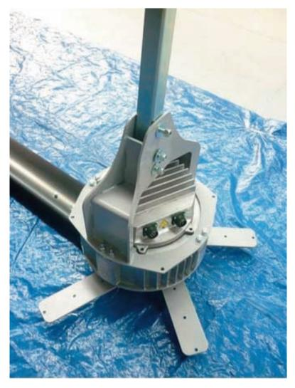
PLACE ROD INTO MOTOR HOLDER AND FIX WITH SCREWS, NUTS AND BOLTS
